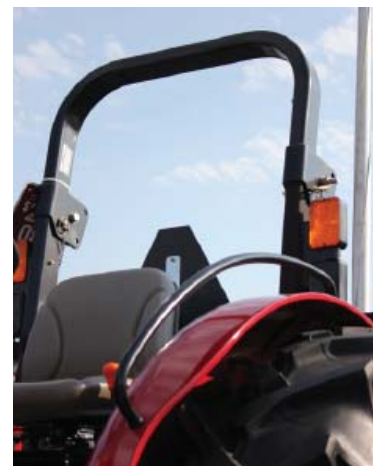
New tractors are manufactured with ROPS. Older models can be retro-fitted with them as well.
